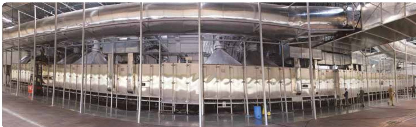
World's largest Onion and Vegetable Dehydration Dryer in terms of length. It has a production capacity of 125 MT per day and is totally Indigenous and manufactured in house, located at Jain Food Park, Jalgaon.
